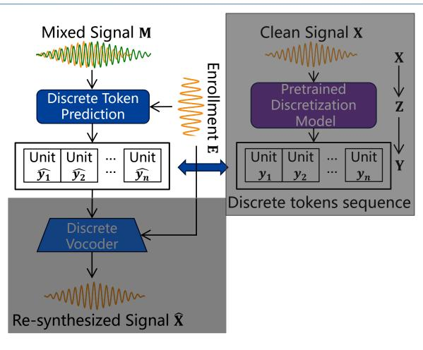
Instead of directly predicting the mask of target speech or mapping the spectrogram, we consider this process as a classification task, where we will predict the discrete tokens frame-by-frame.
