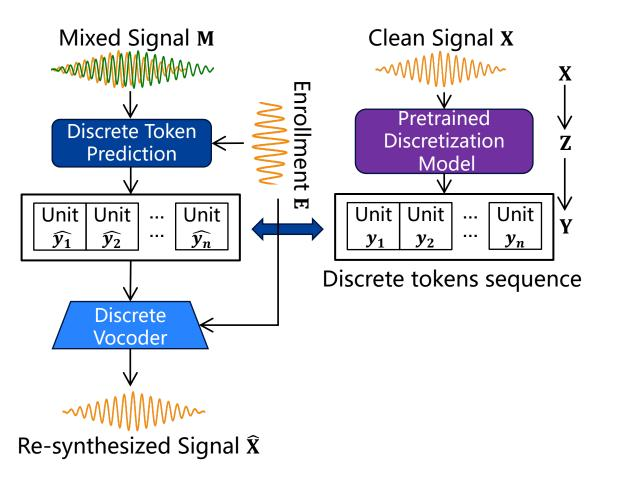
First system to apply a vocoder-based generative method in audio-only TSE.
