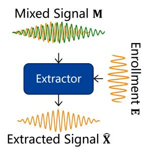
Target speech extraction (TSE) aims at isolating the speech of a specific target speaker from an audio mixture, with the help of an auxiliary recording of target speaker.
