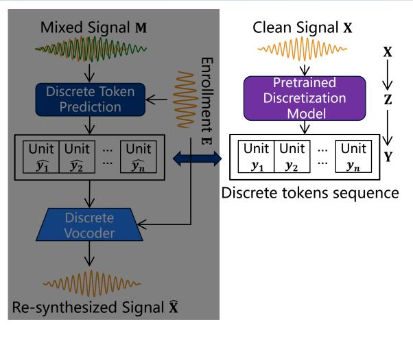
Speech discretization aims to encode the audio input into a discrete sequence.
